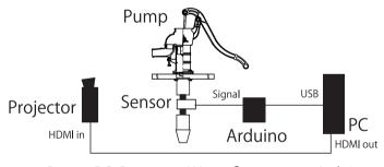
Pump, PC, Projector, Water flow sensor, Arduino This program is written in Unity.
